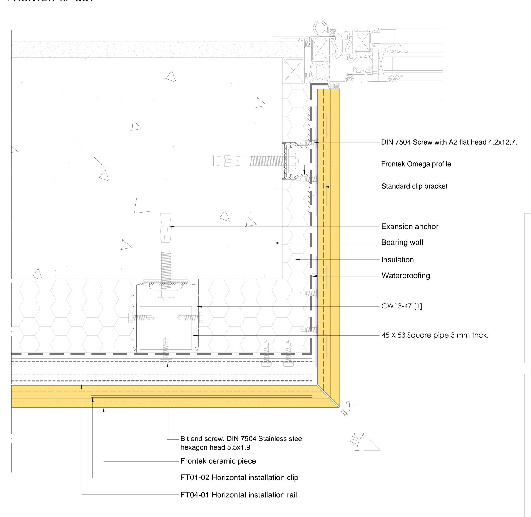
Narrow aluminium section for corner with sealant
