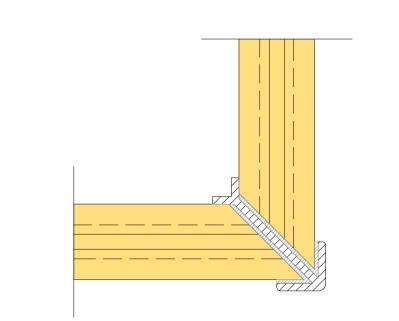
Wide aluminium section for corner with sealant
